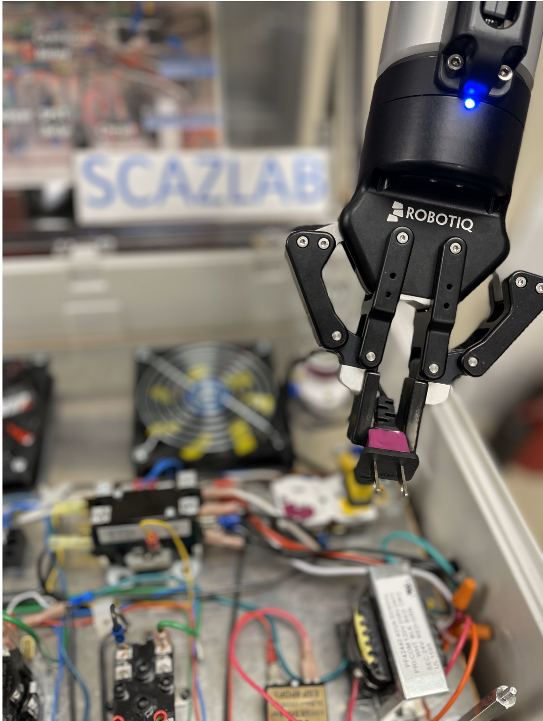
Figure 4.26: Robot unplugs the plug for the compressor so that the participant can measure the resistance at the plug's prongs.
