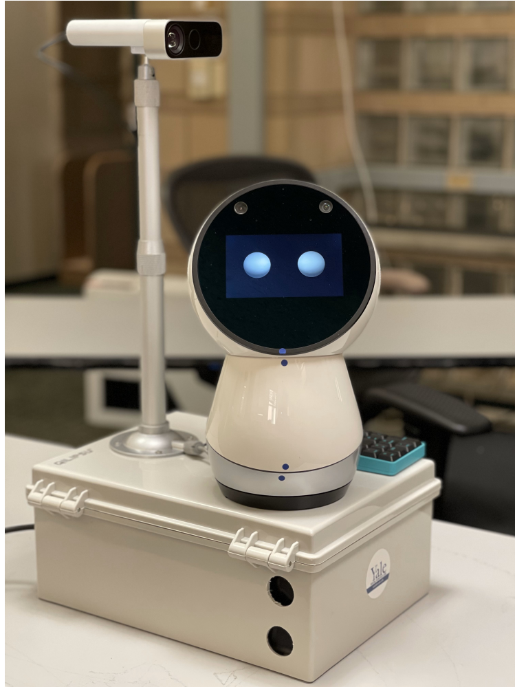
Figure 3.3: Deployable Ensemble - A Jibo robot is attached to a sturdy thermoplastic polymer base box. Also on the base is an Azure Kinect mounted on a mast, and a numeric keypad. Inside the base is a computer, an uninterruptible power supply with surge protection, a network router, and a cooling fan.
