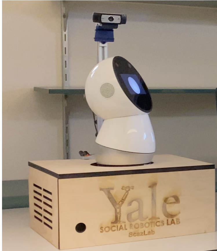
Figure 3.2: Prototype - A Jibo robot is attached to a wooden base. On the base are microphones, a camera, and a toggle switch to power the system on or off. Inside the base is a computer, a battery, a network router, and a cooling fan.
