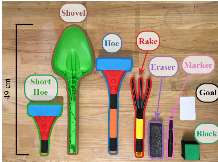
Figure 3.3: The robot had access to 6 tools during our experiments. The tools were used to push and pull a block into a goal region of the workspace. Outlines have been added to color-code each tool and aid in the interpretation of subsequent figures in this chapter.
