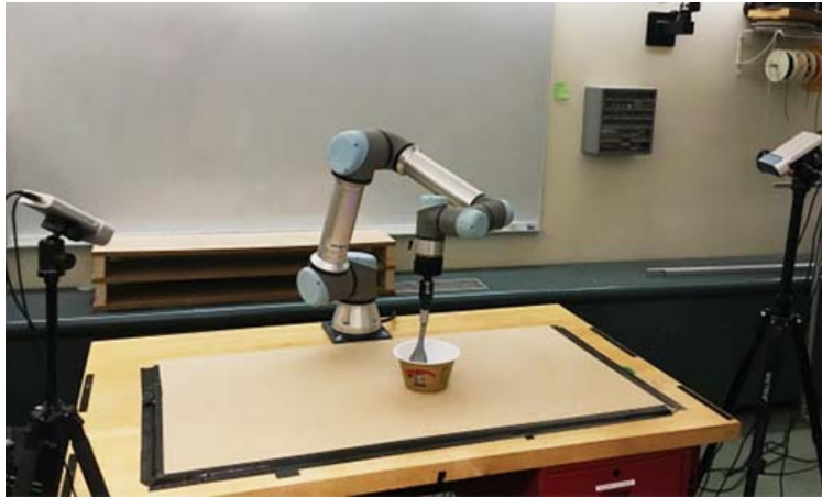
(a) The workspace of the UR5e robot.
