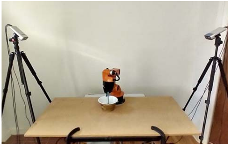
(c) The workspace of the Kuka youBot robot.
