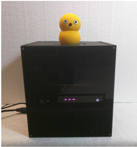
Fig. 3. The MyKeepon robot used in this study is programmed to look at the participant who has most recently spoken, using data from the Microsoft Kinect.
