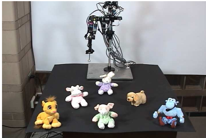
Figure 6.2: During the joint attention experiments, Nico is presented with multiple objects (stuffed animals) with salient colors lying in front of it. Object labels: LL: lion front left, M: pig front middle, RR: genie front right, L: cow middle left, R: dog middle right, B: rabbit in the back.
