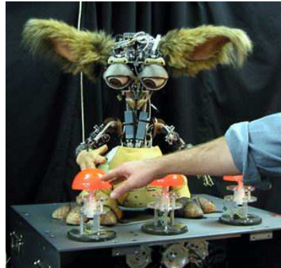
Figure 2.7: Leonardo learns to associate the rightmost button with a label by following the pointing gesture of the experimenter [20].
