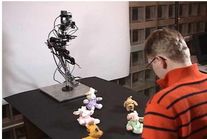
Figure 6.3: Nico points to one of the objects on the table to draw the attention of its caregiver. The caregiver reacts by looking at the object the robot points to.
