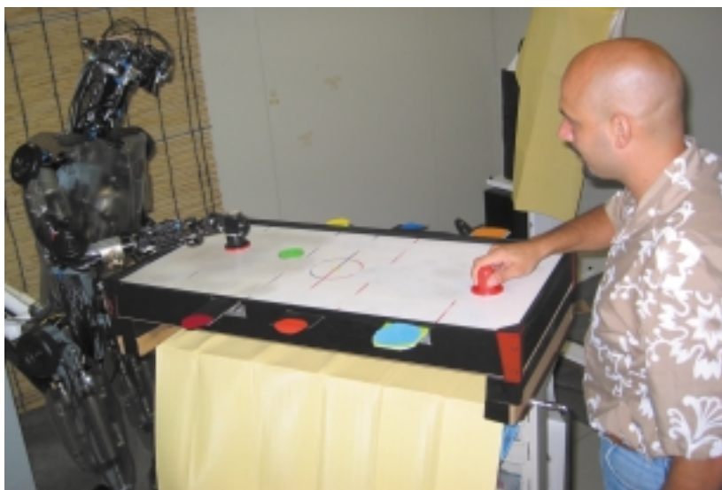
Fig. 1. DB , a full-torso humanoid robot offered commercially by Sarcos, which can learn to play air hockey by observing the movements that a human player makes. The robot's visual system attends to the green puck and the positions of the human player's red paddle. By playing against experienced opponents, the robot learns to position its own paddle to defend its goal successfully and to shoot at the opponent's goal.
