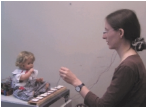
Fig. 4. Robota is a robot doll currently under development at USC. It is able to mimic a few simple gestures of a person wearing infrared markers, such as raising an arm or turning one's head. The demonstrator presses a sequence of keys on a keyboard (each key represents a label such as 'move', 'arm', 'left', etc.), at the same time as performing the corresponding gesture. Using a recurrent, associative neural network, the doll learns the association between the sequence of keystrokes and how they map onto its actions and perceptions of different parts of its body. After training, the demonstrator can press a new sequence of keys without performing the corresponding gesture, and the robot performs it.
