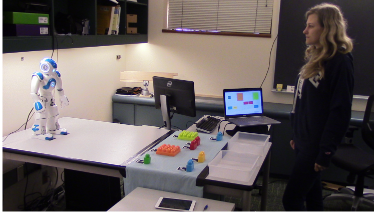
Figure 8.5: The in person evaluation demonstrates the model operating in a real-world human-robot interaction.
