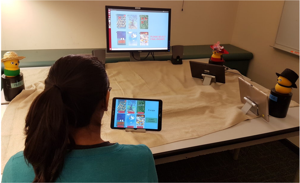
Fig. 1. In this experiment, participants sat around a table playing a game with three myKeepon robots. In certain rounds of the game, the three robots choose a different answer than the one the participant chose. Participants often changed their answers to match the answer of the robots, demonstrating conformity to the group of robots.
