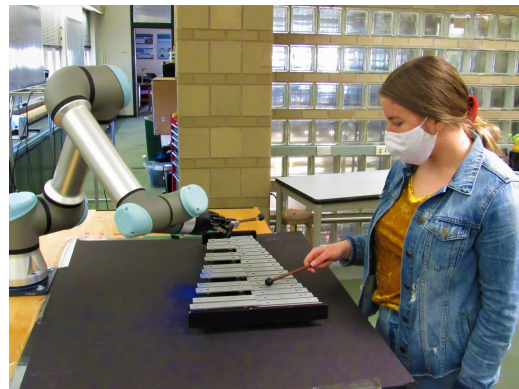
Figure 1: This robot first learns how to play three-note harmonies on a glockenspiel from an instructor, then plays on its own, or with the instructor, and finally becomes the instructor to teach a novice what it has learned.
