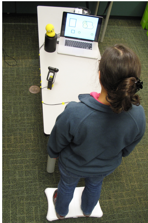
(c) The apparatus viewed from above, Wii Fit Balance Board visible.
