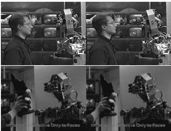
Figure 4: Images captured from a videotape of the robot imitating head nods. The two images at left show the robot imitating head nods from a human caretaker. The output of the face detector is used to drive fixed yes/no nodding responses in the robot. The face detector also picks out the face from stuffed animals, and will also mimic their actions (right images). The original video clips are available at http://www.ai.mit.edu/projects/cog/ .
