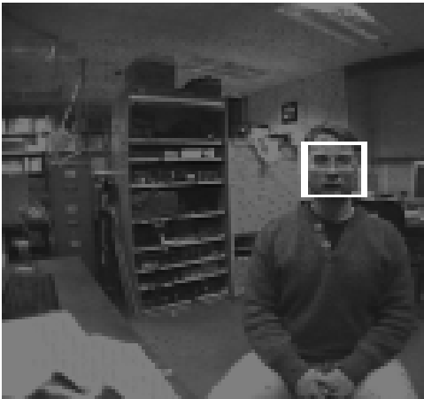
Figure 5: An example face in a cluttered environment. The 128x128 grayscale image was captured by the active vision system, and then processed by the pre-filtering and ratio template detection routines. One face was found within the image, and is shown outlined.
